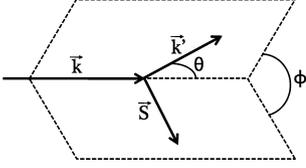
**Fig. 1.** Kinematics for the measurement in the laboratory frame. The electron's initial momentum  $\vec{k}$  and final momentum  $\vec{k}'$  define the scattering plane. The polarization plane is defined by  $\vec{k}$  and the target spin  $\vec{S}$ . The scattering angle is denoted  $\theta$ , while the angle  $\phi$  lies between the scattering and polarization planes.
