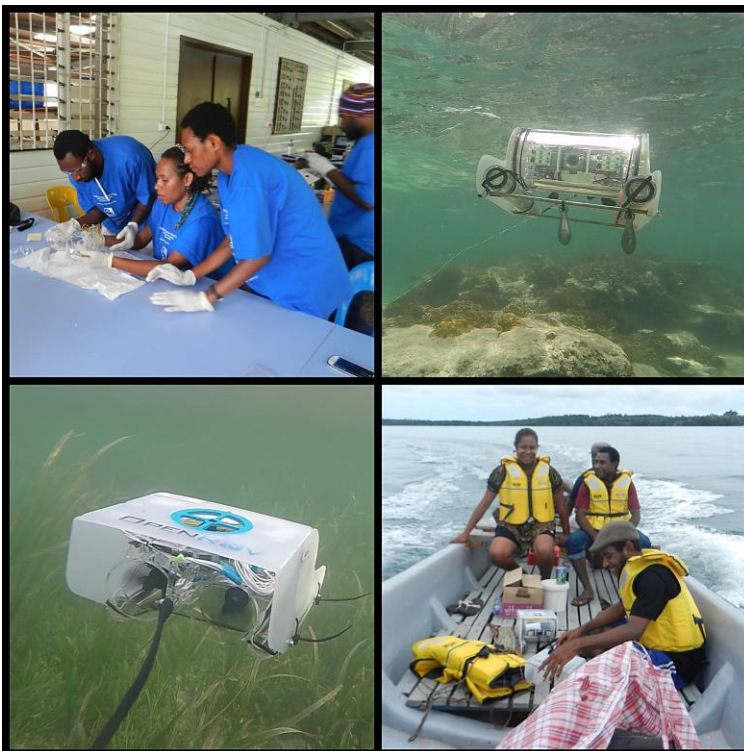
Fig. 1. OpenROV as implemented during the Nautilus Minerals Marine Science Short Course in Kavieng, PNG. Clockwise from top left: Students assemble OpenROV version 2.6 during the MSSC; Forward view of OpenROV version 2.6 in Kavieng Lagoon; Students deploy OpenROV version 2.6 from a small boat in Kavieng Lagoon; Rearward view of OpenROV version 2.6 examining seagrass habitat. Photos by A. Freitag and D. Fretz
