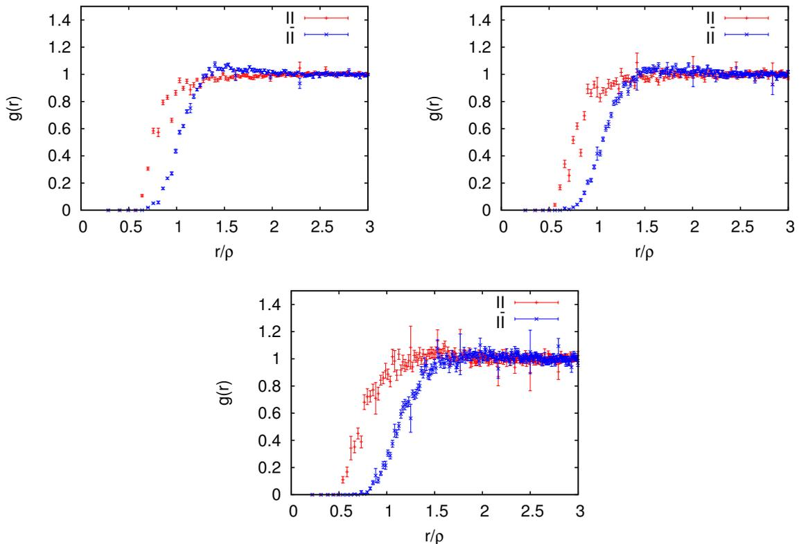
**Figure 3.** (Color online) Pair correlation function for  $II$  and  $AA$  pairs (red) and for  $IA$  pairs (blue) for  $\beta = 4.2$ ,  $V = 32^4$  and a Wilson flow time of  $\tau = 4$  (leftmost upper),  $8$  (rightmost upper) and  $15$  (lower). The distribution is characteristic of a gas, with an excluded volume that is larger for  $IA$  pairs than for  $II$  or  $AA$ .
