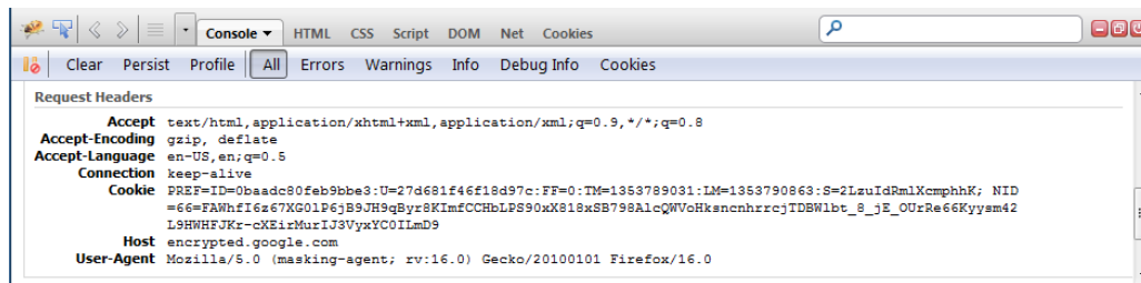
Figure 8: HTTP header request from Google.com (search for “Firefox”)
