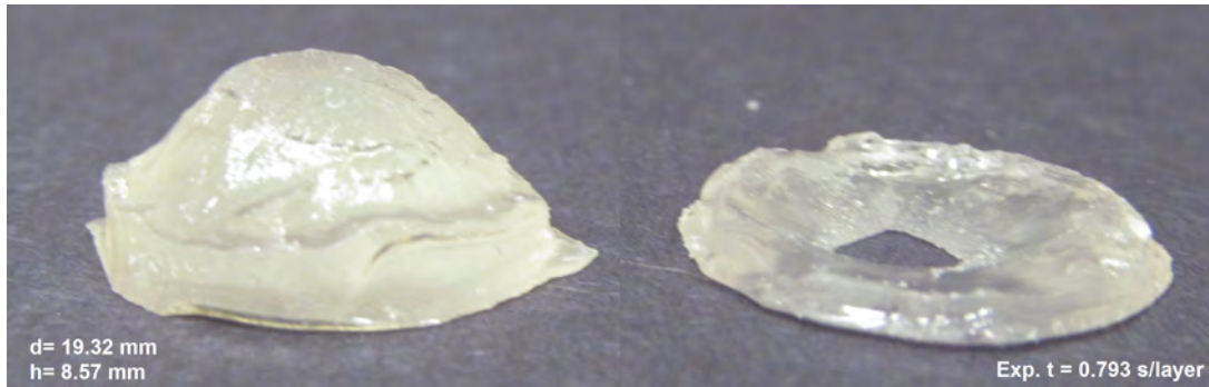
Figure 10: At an exposure time of 0.793 s/layer, this Resin 2.0 print was underexposed. This is evident from the bullet shape of the print (left) and from the size of the ring left on the resin tray, which is roughly the same diameter as the print. If the diameter of the print and the ring are the same, it shows that the ring is part of the build that did not stick correctly to the print and instead built up on the resin tray.
