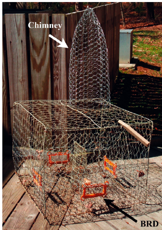
Fig. 2. Crab trap with chimney and bycatch reduction devices (BRD)
