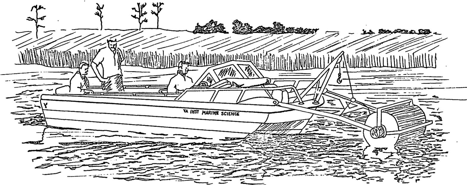
Oil slick samples are obtained by use of a buoyant rotating drum. As the device is pushed along, the surface film adheres to the drum's polished metal surface. As the drum rotates, a stationary blade scrapes the material into a trough from which it is pumped into labeled containers.
