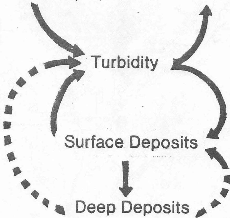
Figure 1. Schematic representation of natural sediment dynamics and how dredging and open water disposal affect these dynamics. Dredging affects are depicted by broken lines. Surface deposits are considered to be on the order of 15 cm in thickness.
