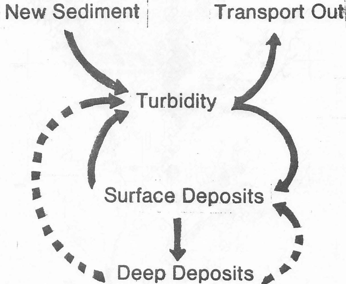
Figure 1. Schematic representation of natural sediment dynamics and how dredging and open water disposal affect these dynamics. Dredging affects are depicted by broken lines. Surface deposits are considered to be on the order of 15 cm in thickness.
