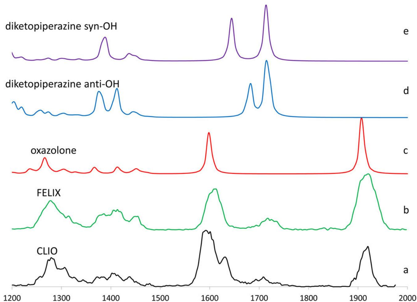
**Figure 1.** Experimental IRMPD action spectrum for  $b_2^+$  ion from PPG obtained at a) CLIO facility and b) FELIX. Computed spectra for c) lowest energy oxazolone conformer, d) lowest energy diketopiperazine structure with *anti*-OH, and e) lowest energy diketopiperazine structure with *syn*-OH.
