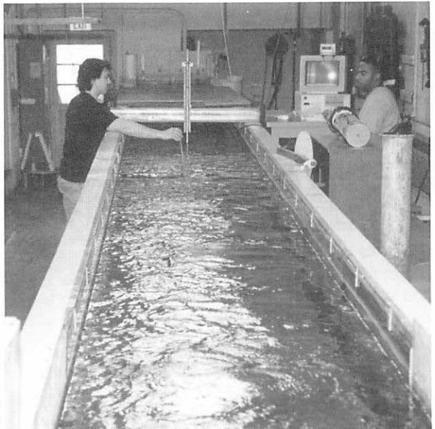
The freshwater flume is used for calibrating instruments before and after deployment.
