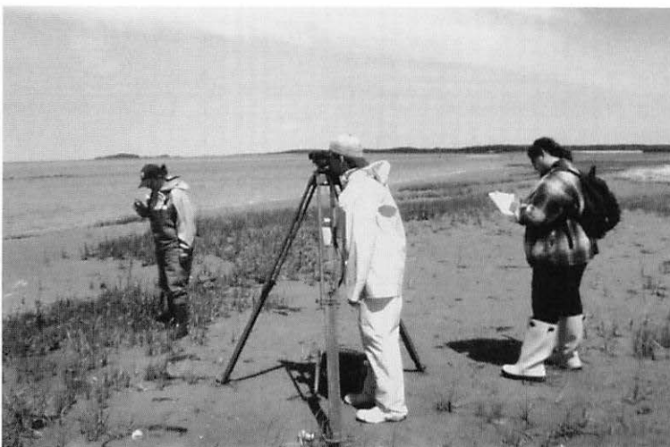
Surveying elevations of constructed intertidal oyster reefs at Fisherman's Island, on the Eastern Shore.
