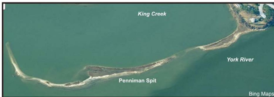
Figure 5-9. Penniman Spit in 2012 (Bing Maps) showing the breach through its middle.
