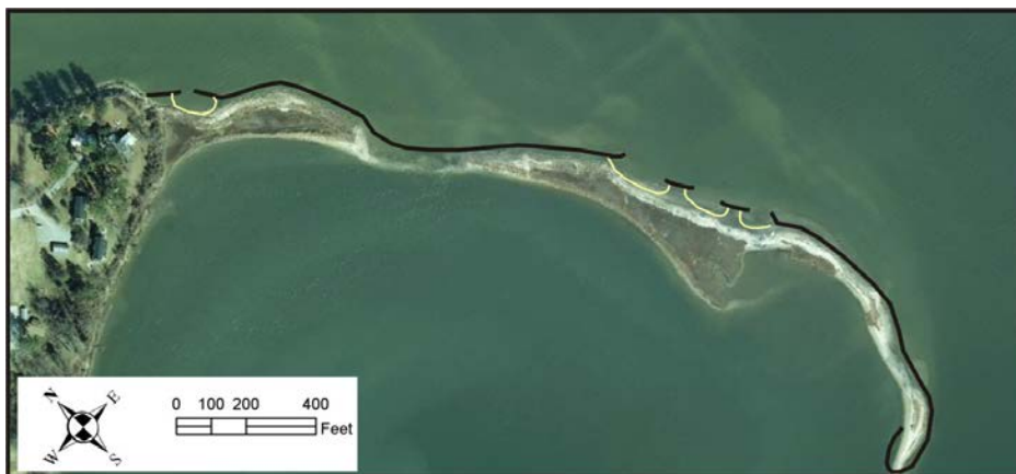
Figure 5-10. Site-specific application of the Shoreline Management Model recommendation for Penniman Spit. The sills will rebuild the spit thereby providing protection the shorelines landward of the spit.
