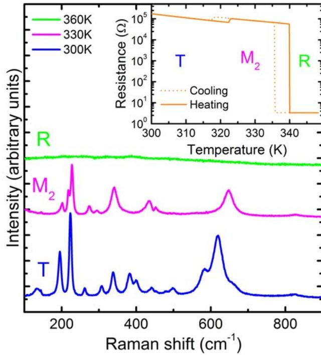
FIG. 2. Raman spectra of a typical  $\text{VO}_2$  crystal studied in our work. Spectra are shown for the T,  $M_2$  and R phases. The  $dc$  resistance of the crystal is plotted as a function of temperature in the inset.
