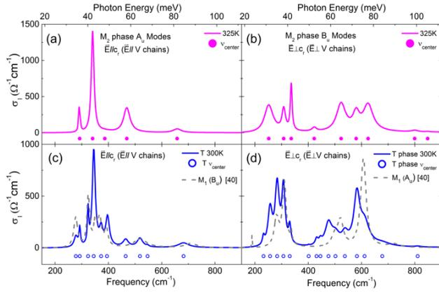
**FIG. 3.** Polarization dependent optical conductivity ( $\sigma_1$ ) showing the infrared active phonon spectra of the  $M_2$  phase (panels (a) and (b)), and the T phase (panels (c) and (d)). The center frequencies of the phonon features are denoted by circles labeled  $\nu_{\text{center}}$ . The previously reported  $M_1$  phase infrared active phonon spectra [40] are compared to the triclinic phase spectra in (c) and (d).
