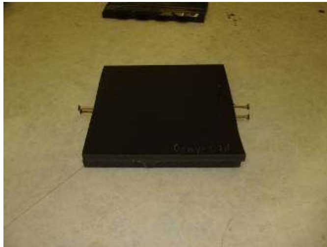
Figure 13: PVC to PVC test sample.
