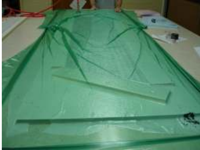
Figure 24: A MINERvA plank sealed under a vacuum bag.
