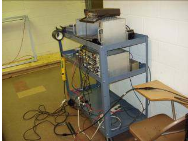
Figure 18: Setup of Test with PMT and pico-ammeter.
