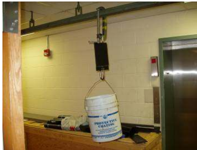
Figure 8: Vertical tension test setup.
