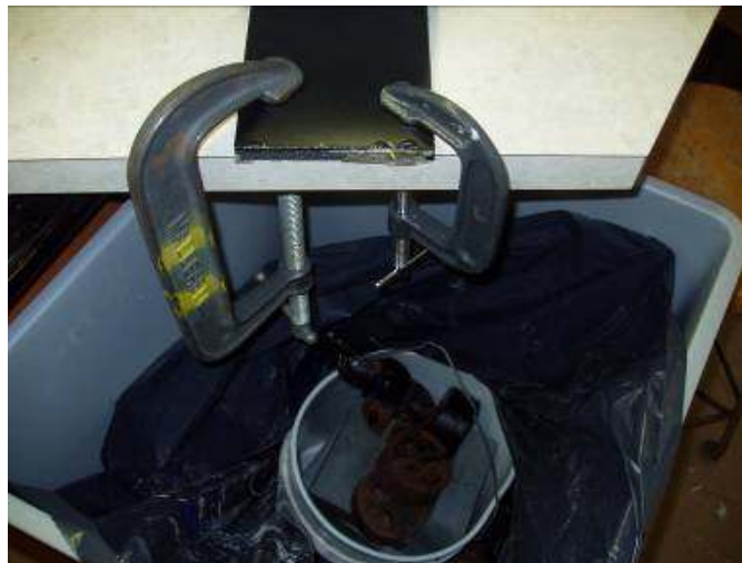
Figure 27: Only the glue was damaged during the translucent epoxy tension tests
