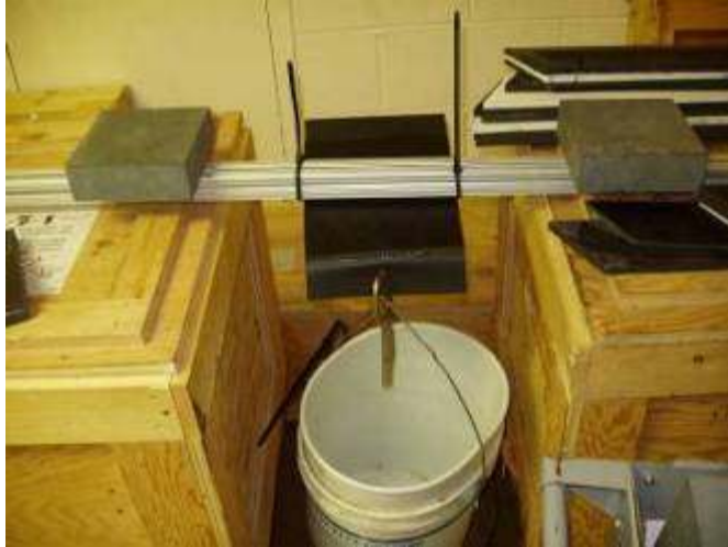
Figure 15: PVC to lexan test setup.
