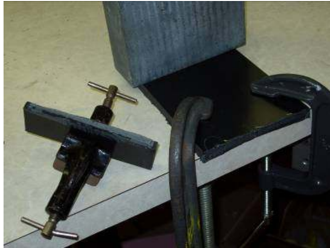
Figure 26: With the gray epoxy, damage was done to the PVC itself when the strip broke.
