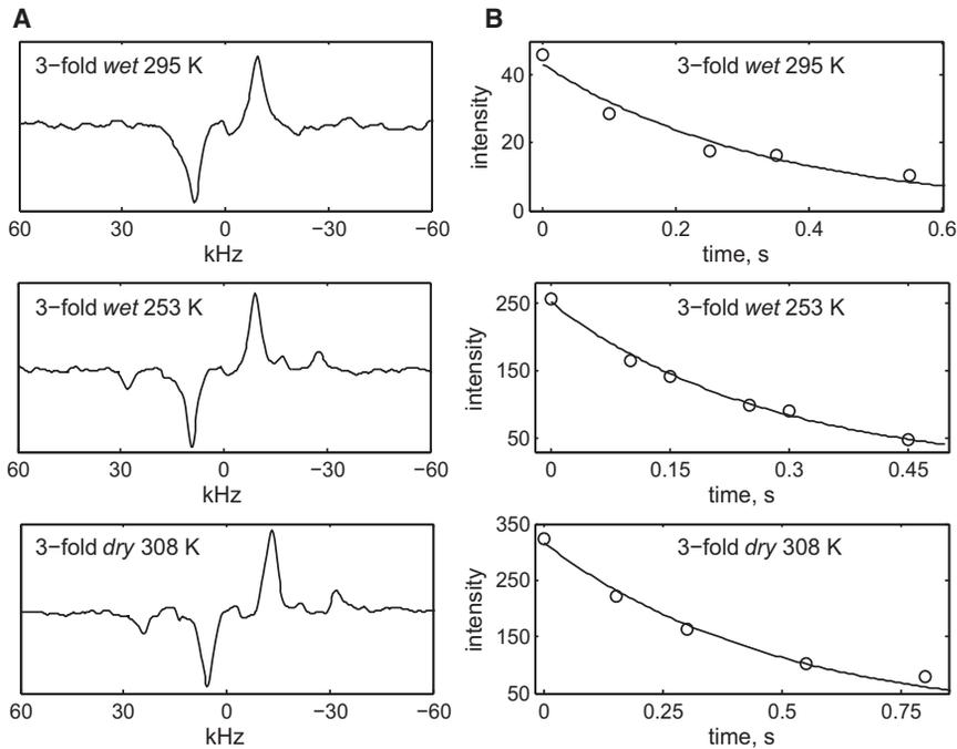
FIGURE 6 (A) Examples of spectra for the  $T_{1Q}$  measurements at the M35 site corresponding to the shortest relaxation delay of 100  $\mu$ s. (B) Corresponding magnetization decay curves at 17.6 T magnetic field strength taken at  $\pm 10$  kHz spikelets are shown. Intensity is shown in arbitrary units.
