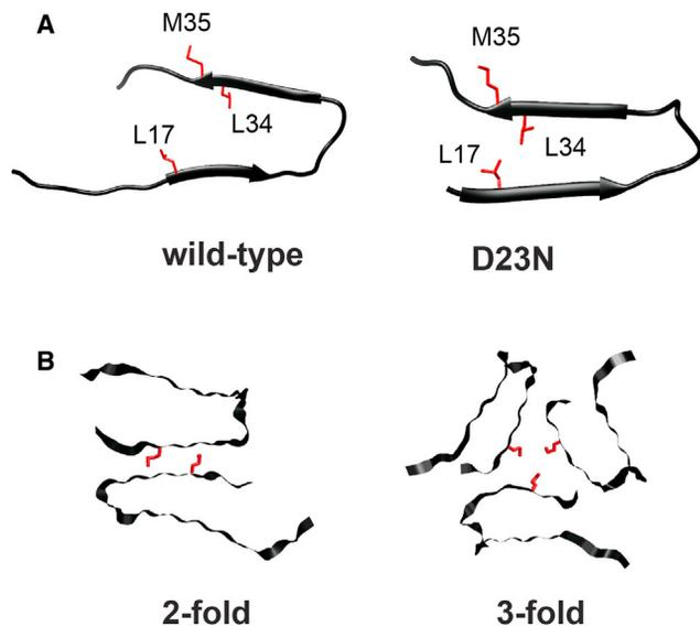
FIGURE 1 (A) Ribbon diagram corresponding to monomeric units of the wild-type  $A\beta_{1-40}$  (PDB: 2LMN, twofold polymorph) and D23N mutant (PDB: 2LNQ), with the side chains investigated in this work in red. (B) Quaternary structures of the twofold (PDB: 2LMN) and threefold symmetric polymorph (PDB: 2LMP) with the side chain of M35 in red are shown. To see this figure in color, go online.
