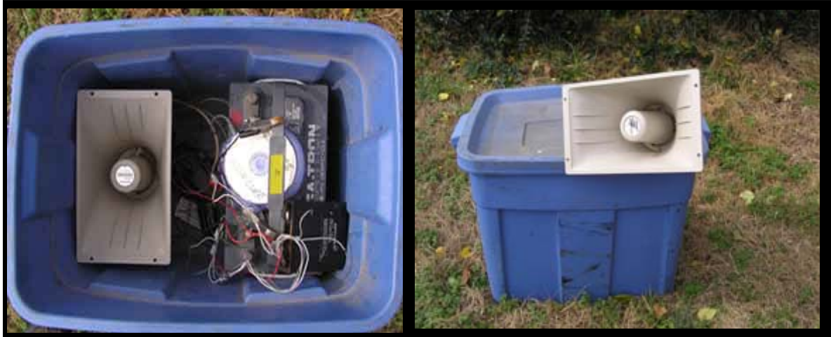
Figure 2. Photos of audio lure components. Photo on left shows components inside plastic container including battery, CD player, amplifier, and bell speaker and connectors. Photo on right shows audio lure in operation with external bell speaker. Photos by Fletcher Smith, CCB.
