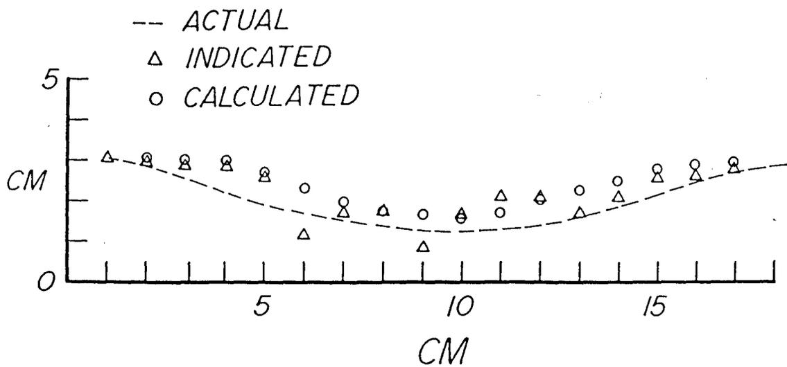
Figure 4. Test of the DSA's ability to delineate a rippled sand bed. The dashed line is the actual ripple profile; the triangles represent the profile indicated by the DSA. The circles represent the profile the DSA would "see" assuming the effective beamwidth of the DSA is 3 degrees.
