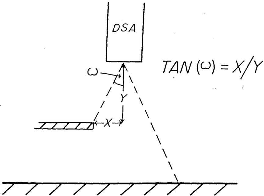
Figure 5. The experimental determination of the effective beamwidth. When the digital output jumps, the plate is in the line-of-sight of the DSA and the beamwidth is calculated.
