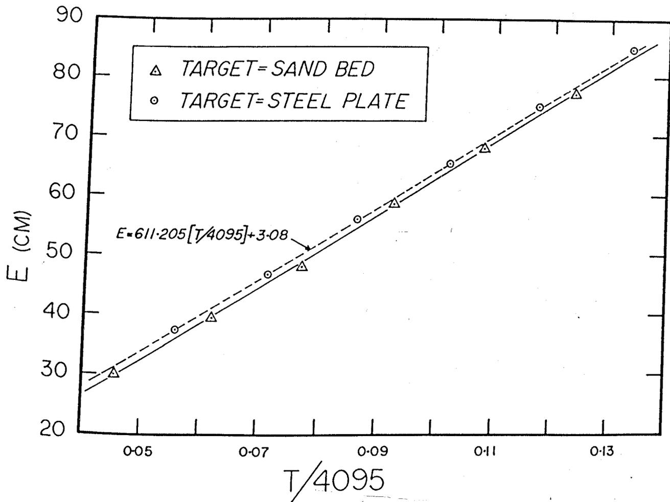
Figure 3. Calibration curve; flat sand bed target.
