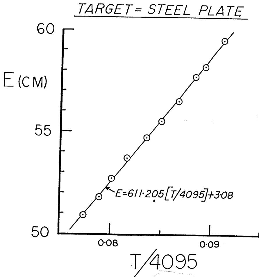
Figure 2. Calibration curve; steel plate target. The DSA is capable of resolving differences in elevation of at least 5 mm.
