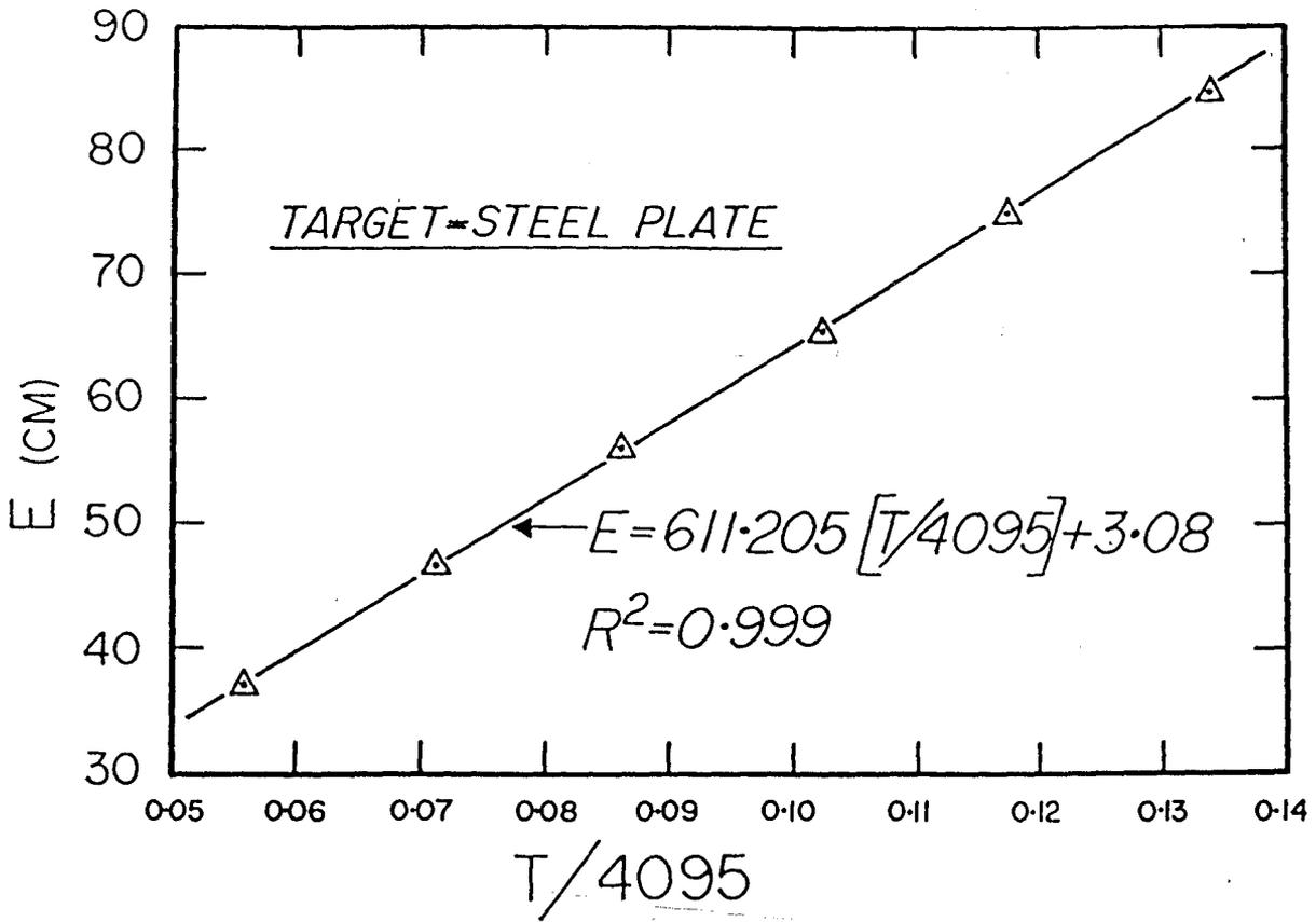
Figure 1. Calibration curve; steel plate target.
