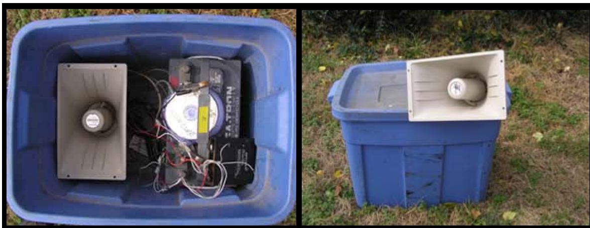
Photos of audio-lure components. Photo on left shows components inside plastic container including battery, CD player, amplifier, bell speaker, and connectors. Photo on right shows audio-lure in operation with external bell speaker. Photos by Fletcher Smith.
