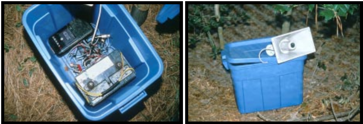
Photos of audio lure components. Photo on left shows components inside plastic container including battery, tape/CD player, amplifier, and connectors. Photo on right shows audio lure in operation with external bell speaker. Photos by Lee Walker.
