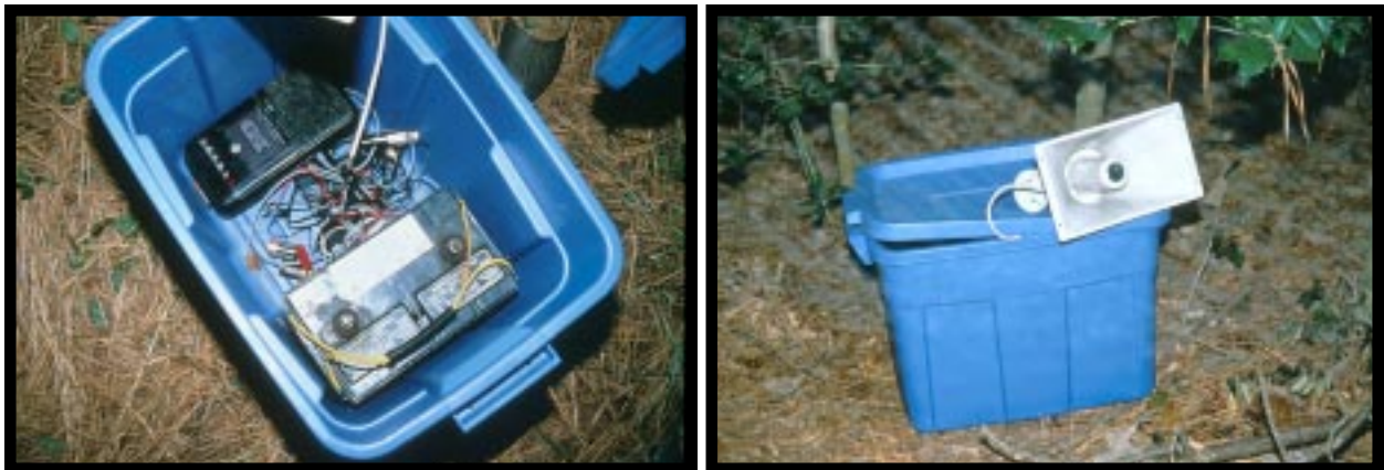
Photos of audio lure components. Photo on left shows components inside plastic container including battery, tape/CD player, amplifier, and connectors. Photo on right shows audio lure in operation with external bell speaker. Photos by Lee Walker.
