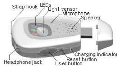
Figure 1: The particular mote used to carry out the experiment on the body sensor network [1].
