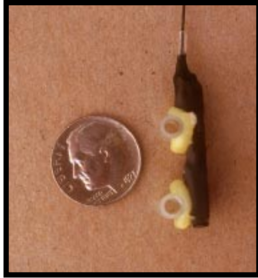
Relative size of Whip-poor-will transmitter. Note harness lugs attached. Photo by Bart Paxton.
