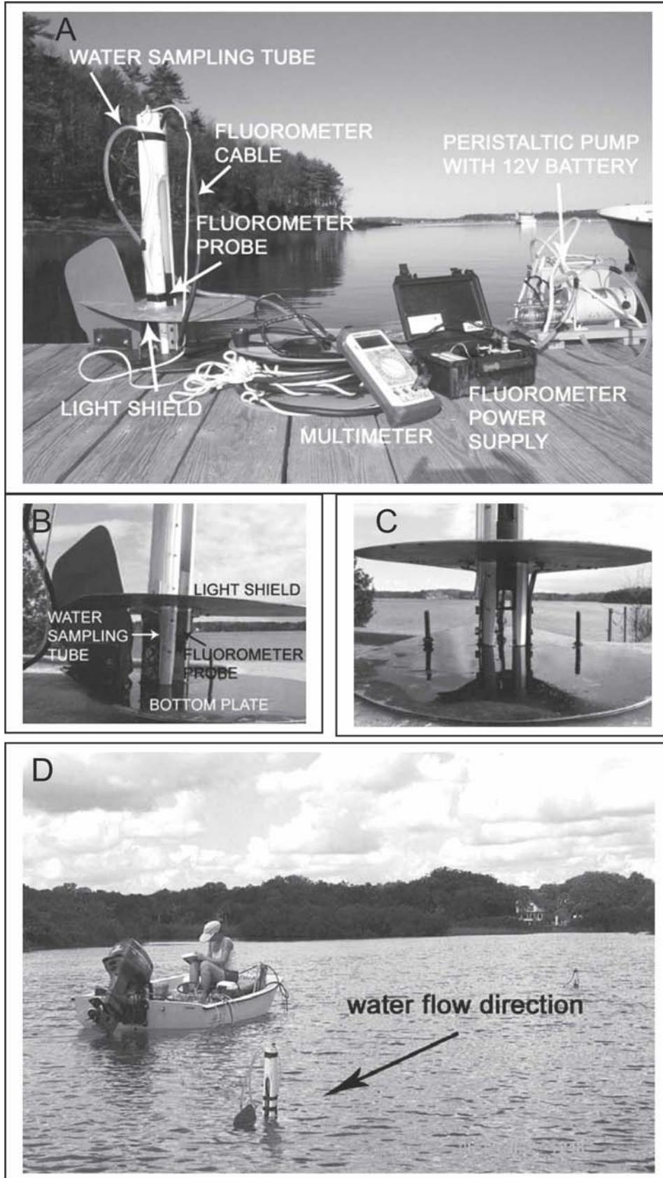
Figure 1. New *in situ* fluorometer and water sampling apparatus. (A) Complete apparatus (one of two identical units); (B) close up oblique view of fluorometer probe in deployment device; (C) close up face-on view; (D) deployment of two identical units over intertidal oyster reef in Florida.
