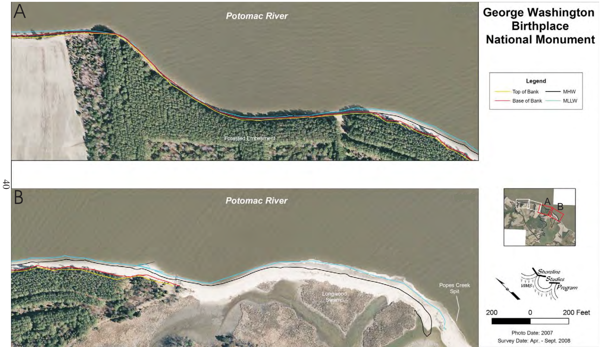
Figure 23. RTK-GPS survey results showing the top of bank, base of bank, mean high water, and mean lower low water along GEWA's eastern Potomac River shoreline.
