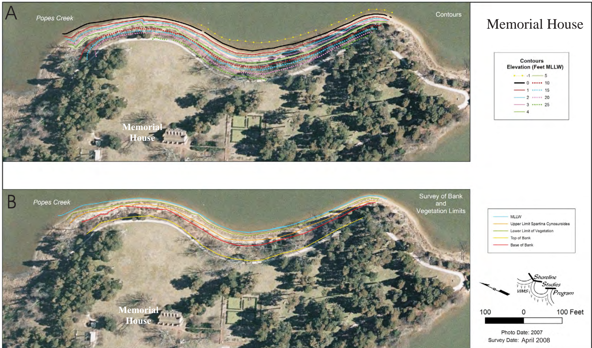
Figure 25. Survey results along GEWA's Popes Creek shoreline at the Memorial House showing A) elevation contours and B) topographic and vegetative features.
