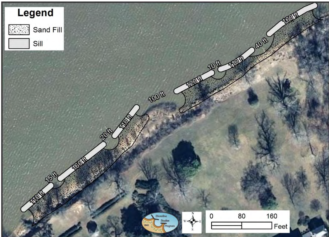
Figure 5-9. Conceptual design of a shore protection system for the eroding shoreline at Upper Brandon on the James River.
