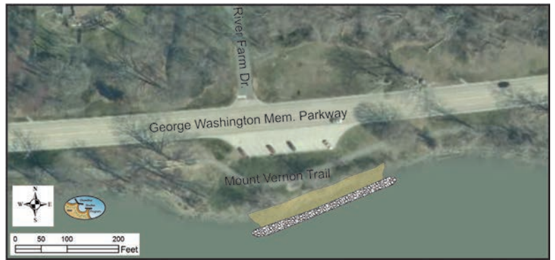
Figure 5-8. Proposed configuration of sill shoreline BMP for Area of Interest #2 along the GWP.
