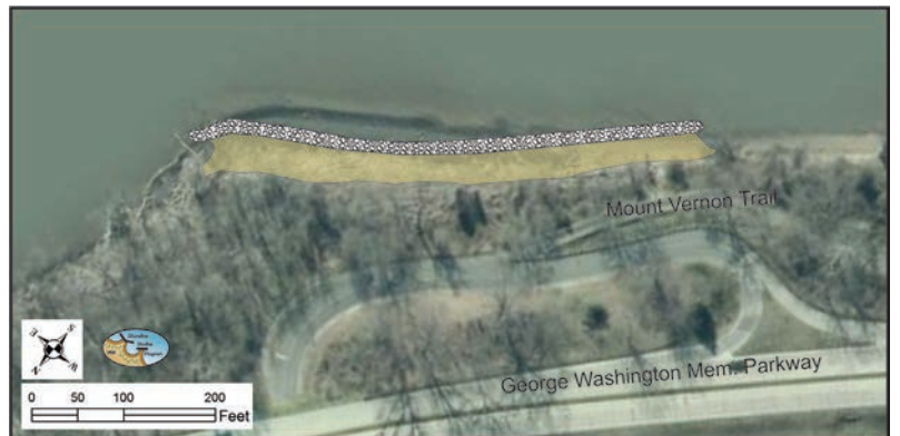
Figure 5-10. Proposed configuration of sill shoreline BMP for Area of Interest #3 along the GWP.
