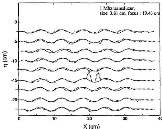
Fig. 8. Comparison of the Averaged Measured Small Ripples (dotted lines) and Background-truth (solid lines) at Different Observation Locations for the 1 Mhz Transducer with Size = 3.81 cm and Focus = 19.43 cm.
