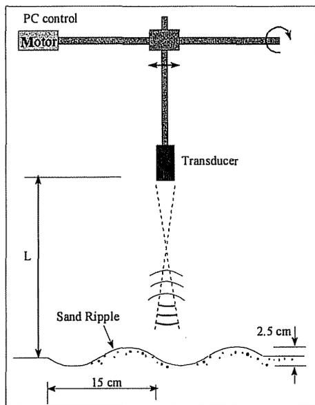
Fig. 2. A Diagram to Show the Experimental Setup.
