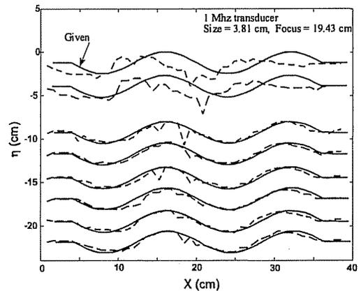
Fig. 6. Comparison of the Averaged Measurements (dashed lines) and Background-truth (Solid lines) at Different Observation Locations for the 1 Mhz Transducer with Size = 3.81 cm and Focus = 19.43 cm for the Large Ripples.
