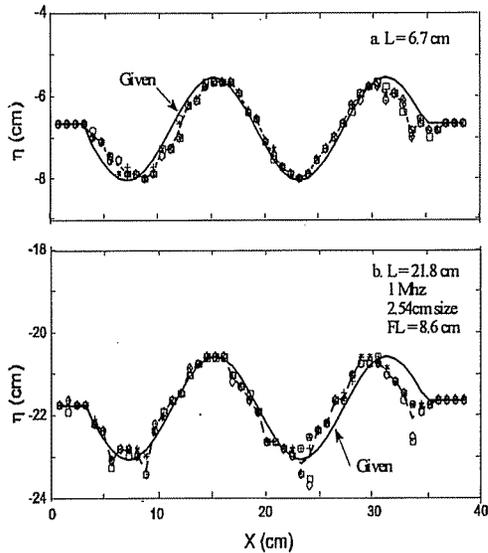
Fig. 4. Selected Results Show the Five Repeated Measurements (the symbols), the Averaged Measurements (the dashed lines), and the Background-truth (Solid lines) using an 1 Mhz transducer with size = 2.54 cm and focus = 8.6 cm. (a)  $L = 6.7$  cm; (b)  $L = 21.8$  cm.
