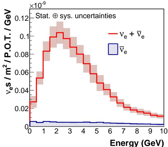
FIG. 1. The  $\nu_e + \bar{\nu}_e$  flux as a function of neutrino energy from the beam simulation for the data used in this analysis. The  $\bar{\nu}_e$  flux is shown separately to emphasize the dominance of  $\nu_e$  in the sum.
