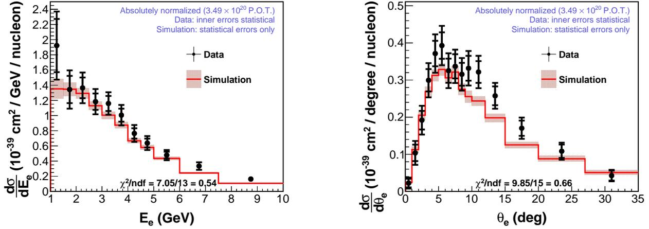
FIG. 3. Flux-integrated differential  $\nu_e$  CCQE-like cross section vs. electron energy (left) and electron angle (right). Inner errors are statistical; outer are statistical added in quadrature with systematic. The band represents the statistical error for the Monte Carlo curve.
