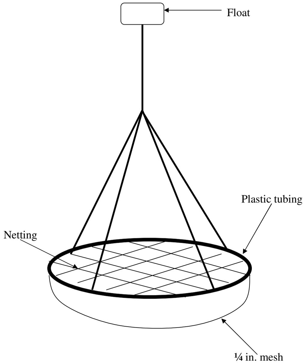
Fig. 1: Basket apparatus used for field sampling. Different volumes of *Gracilaria* spp. were contained in the pocket created by the 1/4 in. mesh. When deployed, the basket laid flat on the sediment surface.
