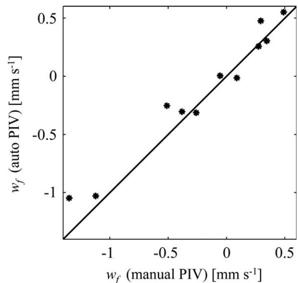
**Fig. 11.** Comparison of mean vertical fluid velocities determined from automatic PIV and manual PIV methods for 11 image sequences.
