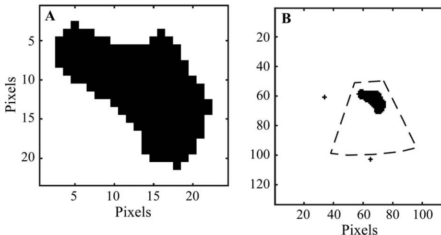
**Fig. 1.** Examples of (A) PTV kernel and (B) target image zones with initial (outer rectangle) and reduced search (dashed region) areas for cross-correlation peak.
