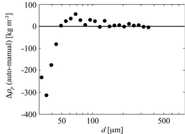
**Fig. 16.** Difference between bin-averaged (by size) particle densities between manual and automatic PIV methods for particle tracking data from Fig. 15.
