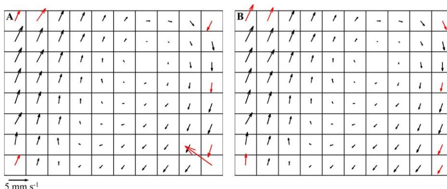
**Fig. 6.** PIV determined velocity vectors. Boxes indicate interrogation areas ( $1.4 \text{ mm} \times 1.3 \text{ mm}$ ) (A) vectors resulting from the PIV cross-correlation, including spurious vectors (red). (B) vectors following spurious vector detection and replacement (replaced vectors indicated in red). Maximum velocity in (B) is  $1.5 \text{ mm s}^{-1}$ .
