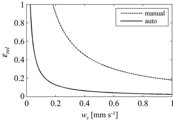
**Fig. 7.** Relative error ( $\epsilon_{rel} = |\delta w_s / w_s|$ ) in settling velocity estimate for manual method (Smith and Friedrichs 2011) and automated PIV method.
