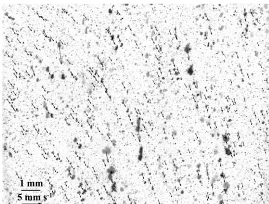
**Fig. 9.** Particle images and displacement vectors from PTV analysis. Particle displacements are indicated from two superimposed image frames (separated by 0.375 s). Particle images are negative representations of the raw images with logarithmic intensity scaling. Particle intensity from the first image is decreased by 25% to better indicate direction of motion. Vector lengths are scaled for display purposes and are not related to the length scale provided.
