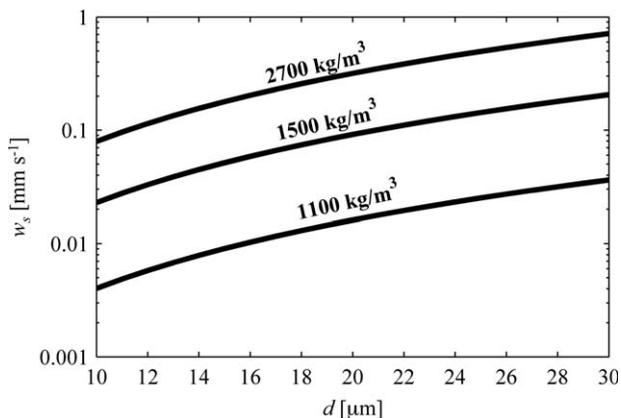
**Fig. 3.** Stokes settling velocity estimate for candidate small-particle diameters and densities.
