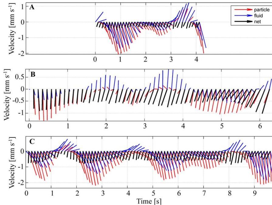
**Fig. 12.** Time-series velocities for three-tracked particles of size (A) 51, (B) 100, and (C) 200  $\mu\text{m}$ . Vectors indicate particle velocity (red), local fluid velocity (blue), and net (settling) velocity (black).
