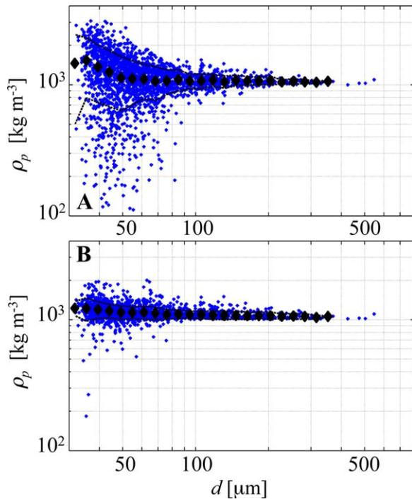
**Fig. 15.** Particle density vs. particle diameter. (A) corrected with mean vertical velocity estimated from 10 manually tracked small particles, (B) corrected with fluid velocities estimated by PIV method.  $N = 2785$  tracked particles, filled diamonds indicate bin-averaged densities for bins with three or more particles, dashed lines indicate  $\pm 1$  SD.
