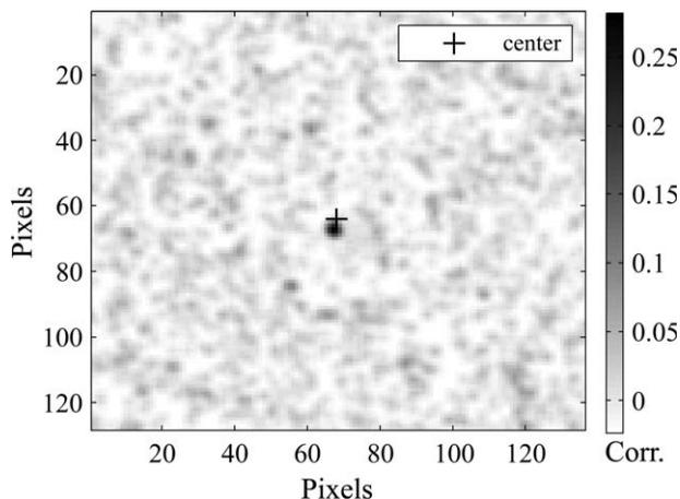
**Fig. 5.** Cross-correlation matrix for interrogation area from Fig. 4. The peak determines the displacement vector of small particles between frames.
