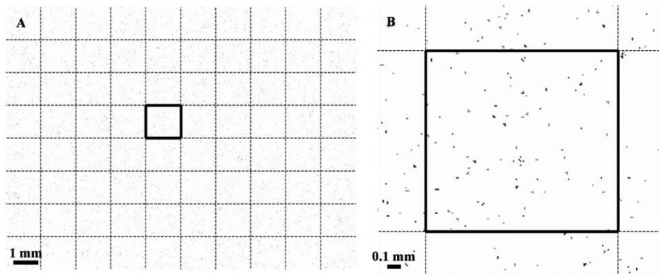
**Fig. 4.** (A) Image with interrogation areas ( $1.4 \text{ mm} \times 1.3 \text{ mm}$ ) for PIV analysis. (B) A single interrogation area (from the bold box in (A)) indicating small particles from two temporally adjacent frames. The lighter-shaded particles are from frame  $l$  and the darker-shaded particles are from frame  $l+1$ .
