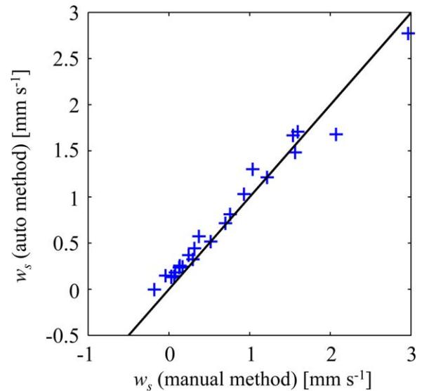
**Fig. 14.** Comparison of bin-averaged settling velocities with manual and automatic PIV methods for particle tracking data from Fig. 13.
