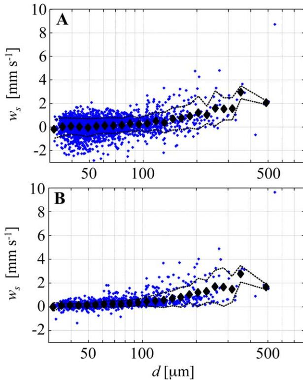
**Fig. 13.** Settling velocity vs. particle diameter. (A) corrected with mean vertical velocity estimated from 10 manually tracked small particles, (B) corrected with fluid velocities estimated by PIV method.  $N=2785$  tracked particles, filled diamonds indicate bin-averaged velocities for bins with three or more particles, dashed lines indicate  $\pm 1$  SD.
