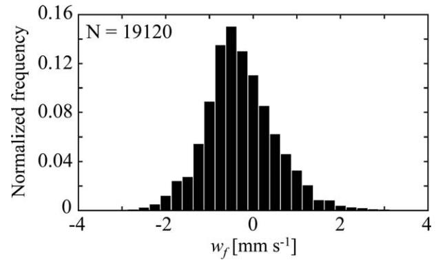
**Fig. 10.** Histogram of vertical fluid velocities from a single image sequence (240 frames). Mean vertical velocity is  $-0.305 \text{ mm s}^{-1}$  (downward).
