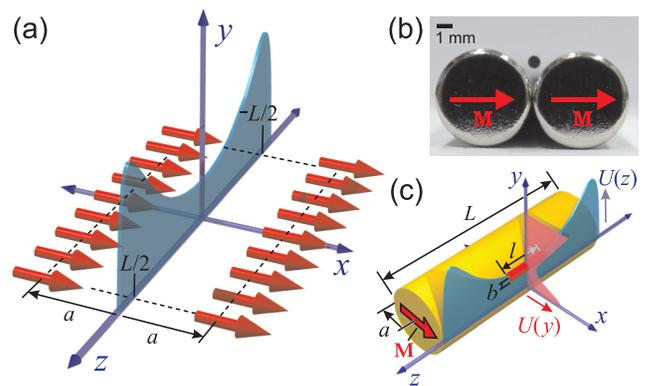
FIG. 1. The PDL system and its experimental realization: (a) The PDL model that produces a camelback potential at the center plane for  $|y| < a$ . (b) Experimental realization with diametric magnet pair system that serves as magnetic trap for a diamagnetic (graphite) rod. See the supplementary material A (Ref. 16) for detailed system parameters. (c) Schematic diagram of the PDL trap with only one magnet shown.
