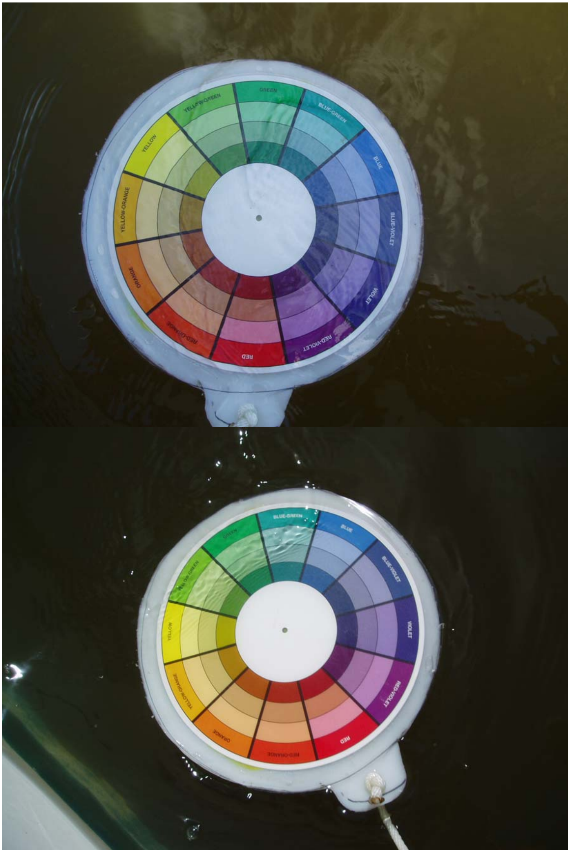
Figure 3-17. High Angle Water Color Photography; December 14, 2004; Sunny Mid-day; Shade Side (top); Sunny Side (bottom)
