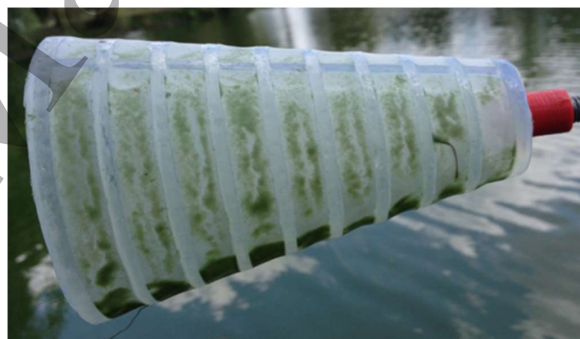
Figure 16: Real algae has been collected in the field and initial deposition patterns suggest that cross-step filtration is working as expected. Field observations of real algae accumulation on the mesh will be challenging to obtain.
