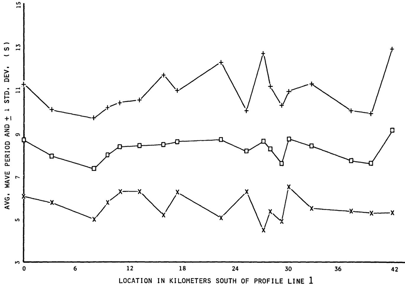
Figure 20. Average breaker period at the 18 survey locations based on 25 observations at each profile location (1974-1976).
