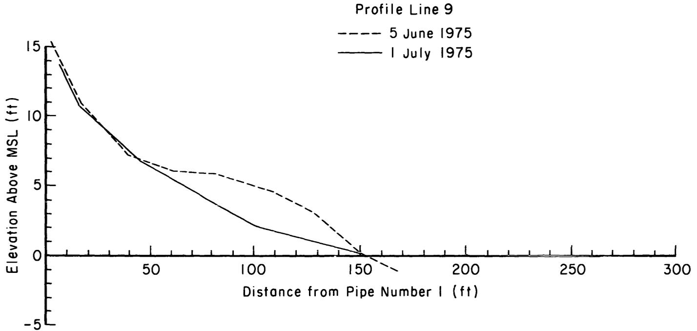
Figure 22. Typical profiles at narrow beach showing both accretional (5 June 1975) and erosional (1 July 1975) shapes. Compare with changes at profile line 1 during same period (Fig. 21).
