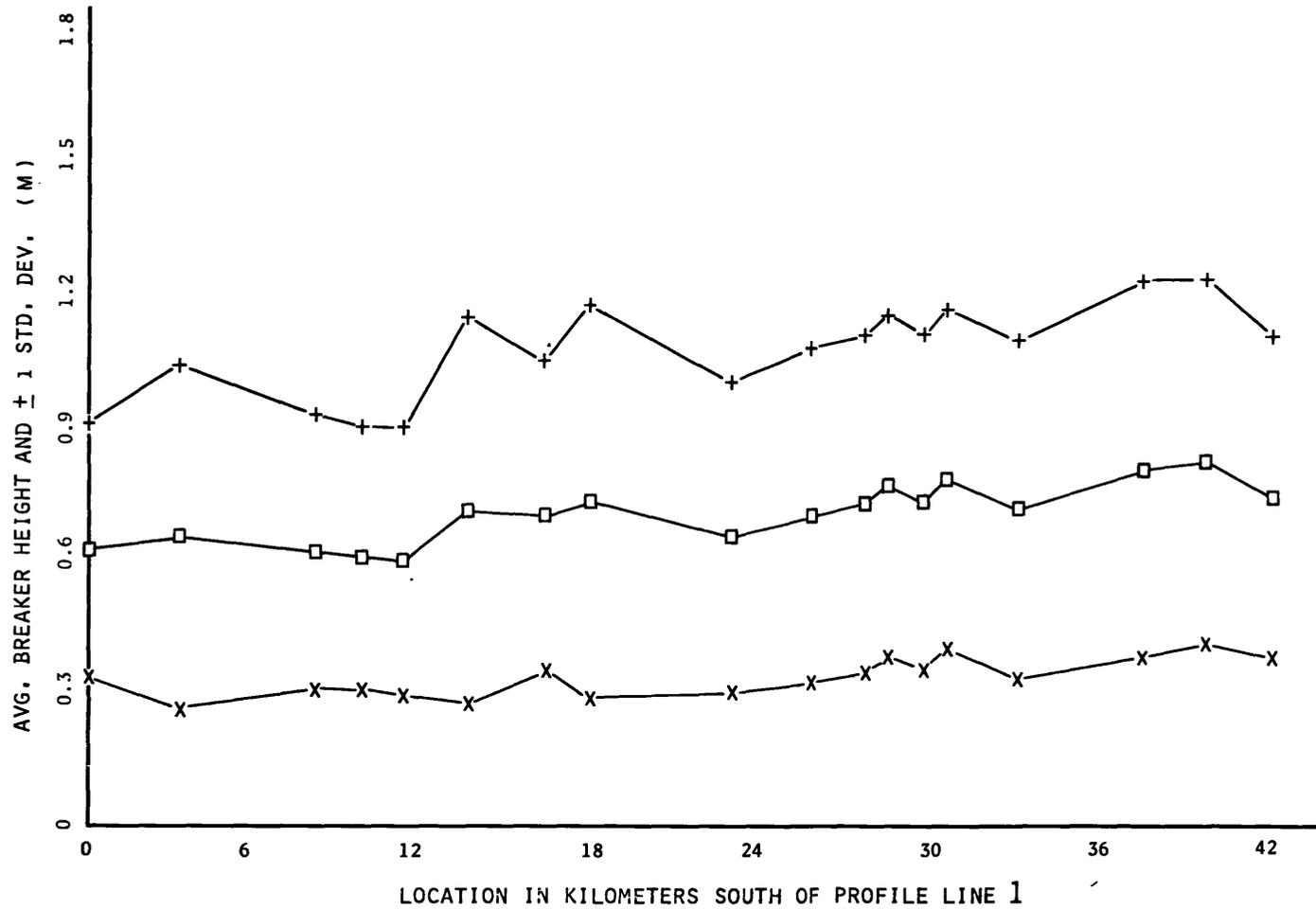
Figure 19. Average breaker height at the 18 survey locations based on 25 observations at each profile location (1974-1976).
