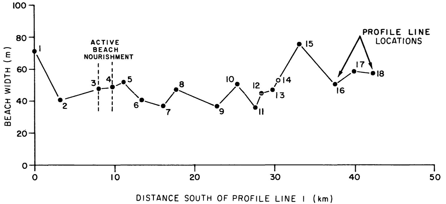
Figure 23. Mean beach width at 18 profile lines, September 1974 to November 1976. "Beach width" is from mean sea level to the base of the dune, or equivalent.
