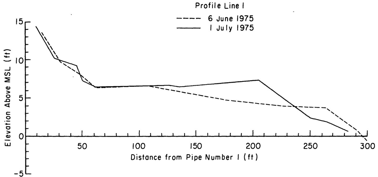
Figure 21. Typical profiles at wide, accreting beach showing both accretional (6 June 1975) and erosional (1 July 1975) shapes. Dropoff at seaward end due to channel.
