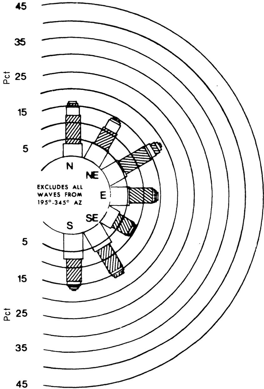
Figure 10. Ship observation wave rose (from Gutman, 1976).
