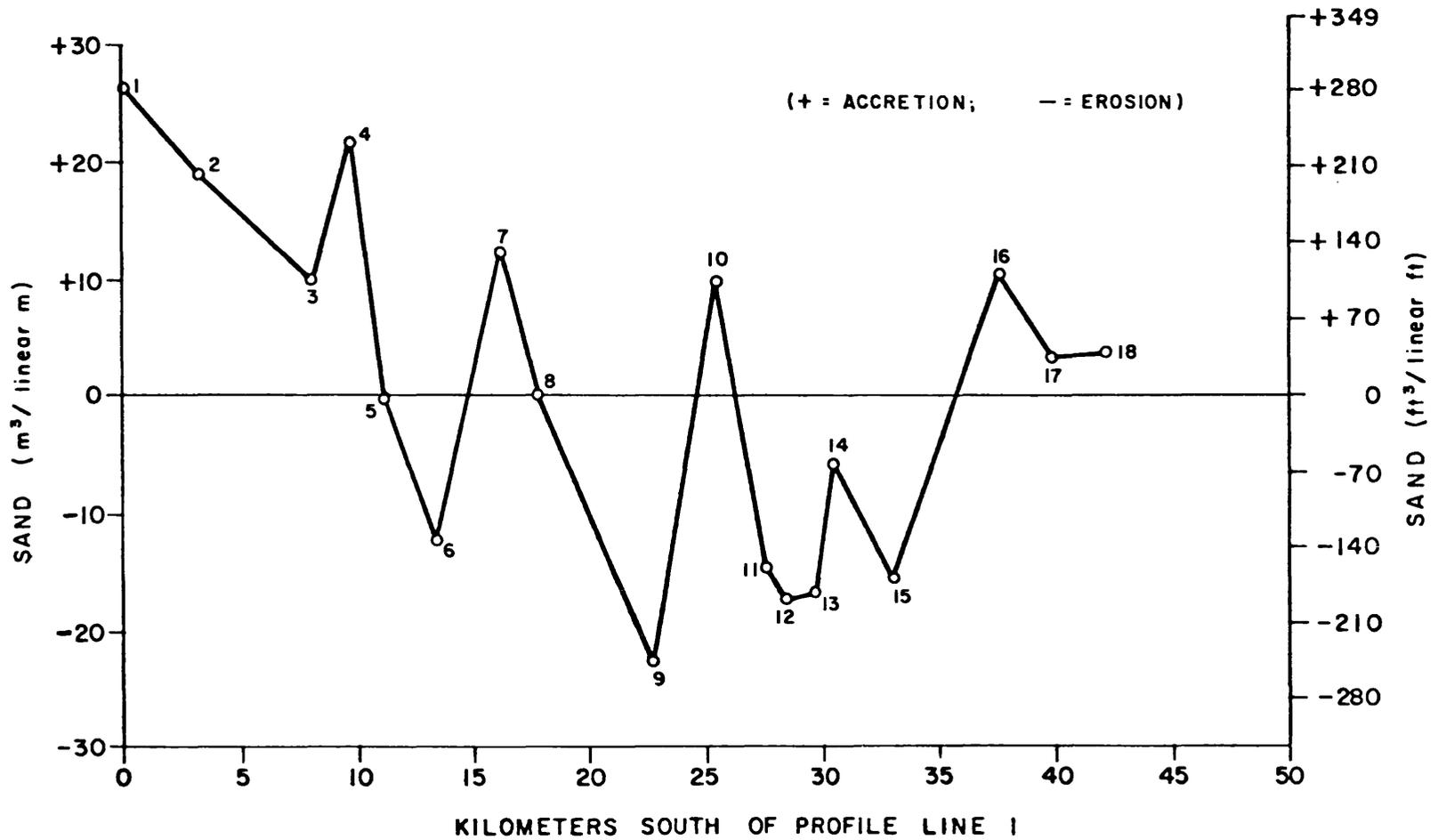
Figure 13. Cumulative beach volume change at 18 profile locations, September 1974 to November 1976. Numbers 1 to 18 on volume line indicate the profile lines.
