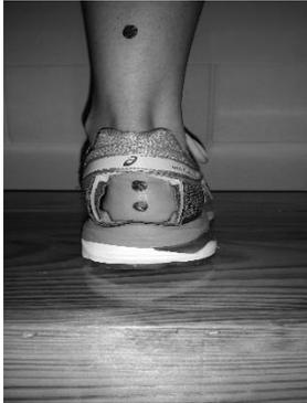
Figure 4. Heel window in right shoe with vertical calcaneus markers.
