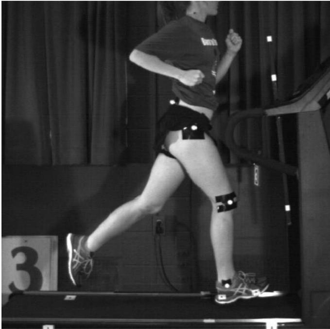
*Figure 6.* Markers captured by the side view camera.
