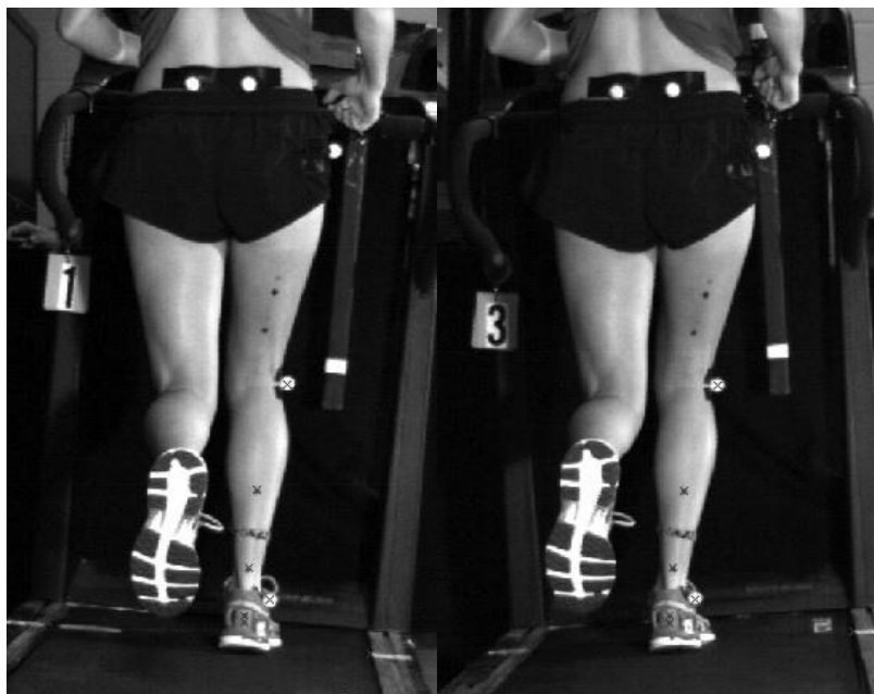
Figure 1. Medial elevation (ME) was created by raising the left side of the treadmill by 5°, (photo on left) and lateral elevation (LE) was created by raising the right side of the treadmill by 5° (photo on right).
