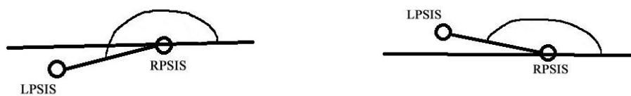
Figure 9. Lateral pelvic tilt left (on the left) (angle greater than 180 degrees), lateral pelvic tilt right (on the right) (angle less than 180 degrees). Markers on the left PSIS (LPSIS) and the right PSIS (RPSIS).
