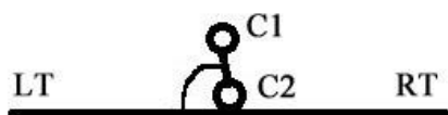
Figure 13. Rearfoot with respect to treadmill, two markers on the calcaneus (C1 and C2), and two markers on the left (LT) and right (RT) sides of the treadmill, a smaller value indicates greater eversion.
