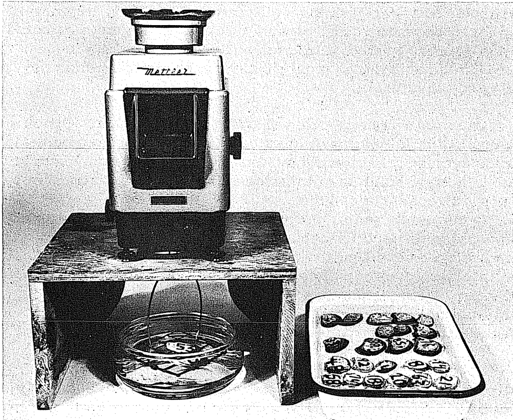
Fig. 1. Arrangement of Mettler scale for suspension weighing in water. Suspension equipment is tared permitting direct reading of oyster weights.
