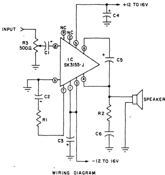
FIGURE 2. Details of the amplifier system and speaker.
