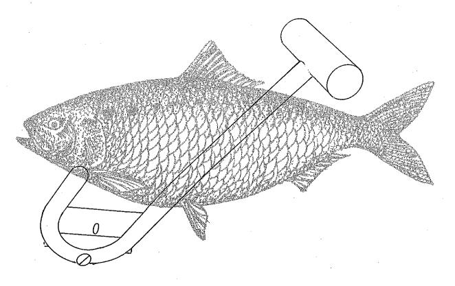
A KNIFE DESIGNED EXCLUSIVELY for opening fish for roe removal may prove a boon to shad processors, in light of preliminary tests. The new knife is faster and more efficient to use than a conventional knife, and because of its unique blunt-end design, poses less of a threat to the fragile roe.
