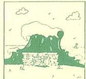
The traditional use of vertical bulkheads to protect shorelines from erosion or to protect perimeters of boat basins can create problems.
