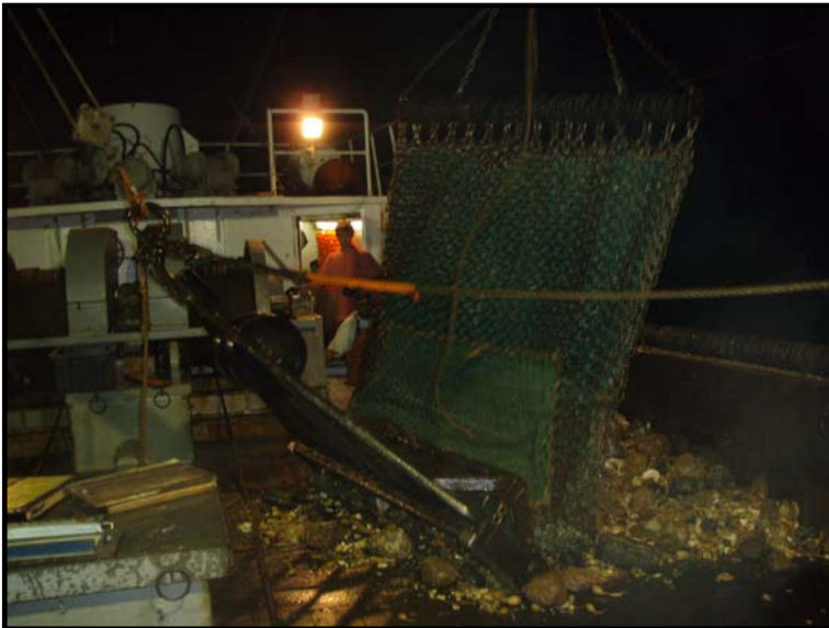
Figure 4 “Prototype” sea scallop survey dredge as developed by the Scallop Survey Advisory Panel (SSAP).
