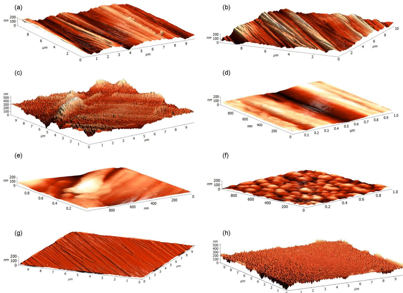
**Fig. 1.** Atomic force microscopy (AFM) images of control (a and d), RFGD-treated (b and e), and heat-treated (c and f) Ti-6Al-4V for  $10\ \mu\text{m} \times 10\ \mu\text{m}$  scan area (a–c) or a  $1\ \mu\text{m} \times 1\ \mu\text{m}$  scan area (d–f). After applying a spatial high-pass filtering with a 200 nm-cutoff to (b) and (c), respectively, only the small-scale features of the RFGD-treated (g) and heat-treated (h) samples remain.
