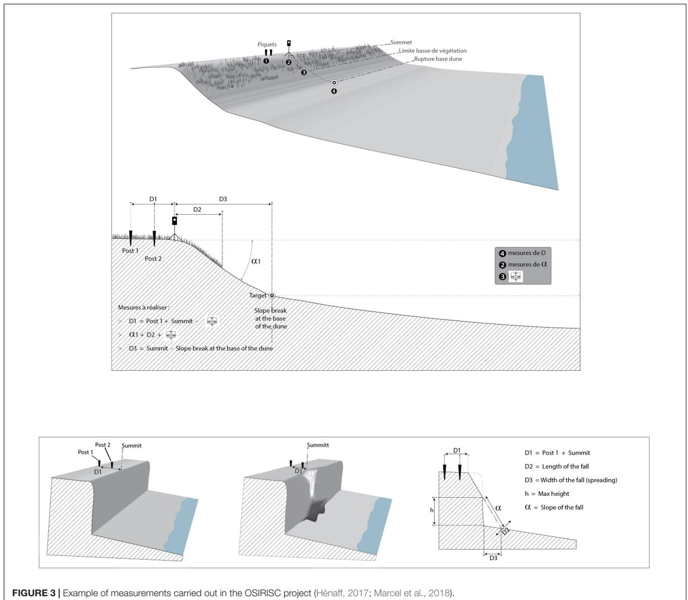
**FIGURE 3** | Example of measurements carried out in the OSIRISC project (Hénaff, 2017; Marcel et al., 2018).
