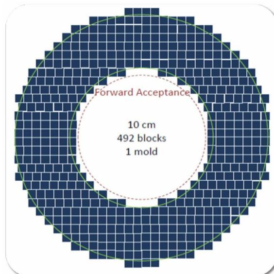
Figure 4. The layout of SIDIS large angle calorimeter with square modules.
