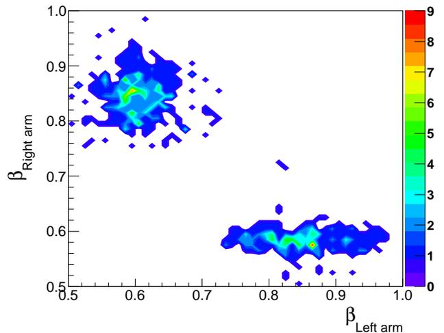
FIG. 1. (Color online) The  $\beta$  distribution of particles detected in coincidence by the two High Resolution Spectrometers in Hall A/E03-101. The widths of the peaks result from the calibration and time resolution of the scintillators, from the momentum acceptance of the spectrometers ( $\Delta p \approx \pm 3.5\%$ ), and the uncertainty of the path-length correction. The different scintillators in the two spectrometers lead to different widths of the distributions.
