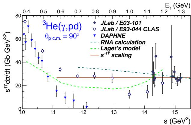
FIG. 3. The invariant cross section  $d\sigma/dt$  multiplied by  $s^{17}$  to remove the expected energy dependence. The DAPHNE data is taken from [28]. The RNA [18] calculation is normalized to our highest energy data point from JLab/E03-101. The prediction of Laget is based on a diagrammatic hadronic model [38]. Constant  $s^{17}$  scaling normalized to our highest energy data point is indicated by a solid red line. For a comment on the comparison between the CLAS and DAPHNE data see [39].
