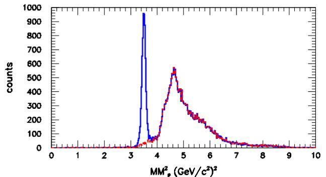
FIG. 2. (Color online) Event distributions measured by CLAS, of the missing-mass of the proton,  $MM_p^2$ , for  $\theta_{p\text{ c.m.}}=90^\circ$ , with (dashed red line) and without (blue solid line) the kinematic cuts, are shown. Events from the  $pd$  final state are clearly identified in the peak. The background distribution (events rejected by the kinematic cuts) exhibits smooth behavior under the deuteron peak and reproduces the background shape outside of the peak.
