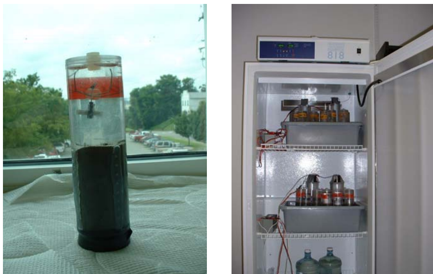
Figure 6. Small sediment core used for mineralization with magnetic spinner inside core (left). Small sediment cores placed around large magnetic spinner in temperature-controlled incubator (right).
