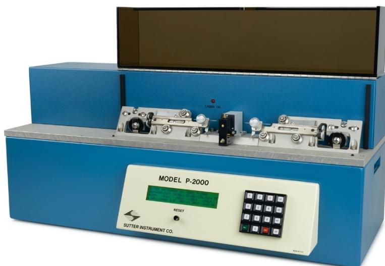
Figure 2.5 Sutter P2000 pipette puller. The black object in the center of the assembly is the housing for the laser. The mechanism on either side is the arms that hold and pull the capillary into the needle shape.<sup>33</sup>
