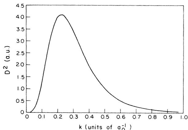
FIG. 2. Variation of the square of the bound-free radial matrix element with ejected electron momentum.
