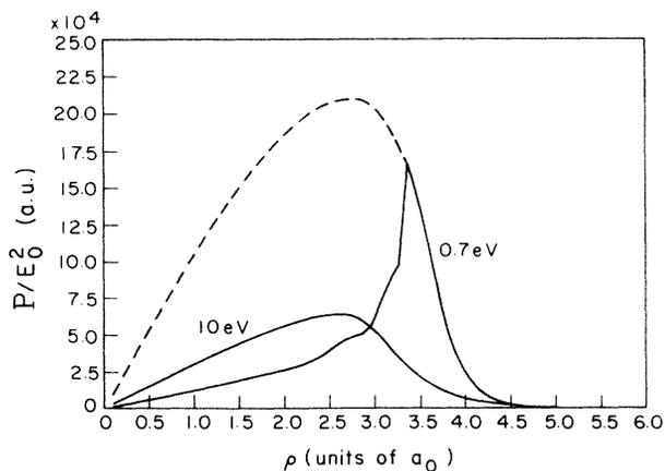
FIG. 3. Variation of total LICD probability ( $P/E_0^2$ ) with impact parameter. The dashed curve shows the 0.7-eV result for uninterrupted straight-line paths.
