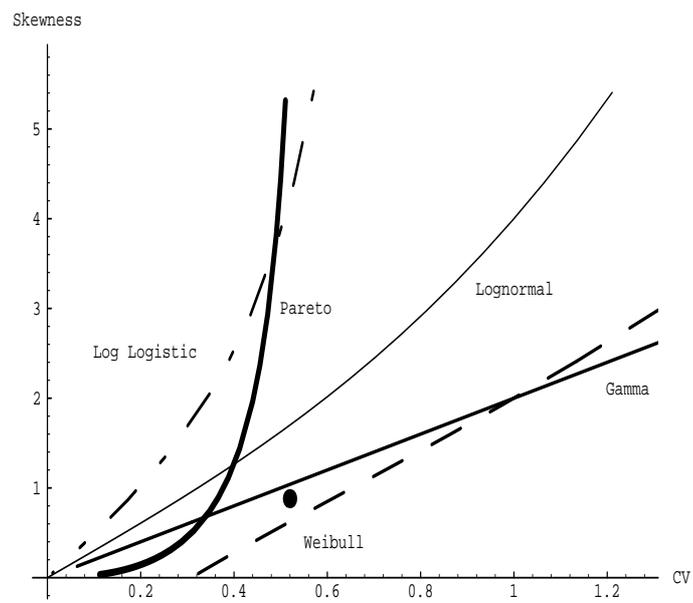
Figure 7: Skewness vs. Coefficient of Variation [Ball Bearings at (0.52, 0.88)]
