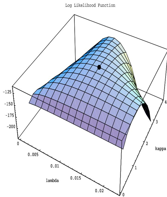
Figure 4: Log Likelihood Function with Maximum Value Identified (Ball Bearings, Weibull Fit)
