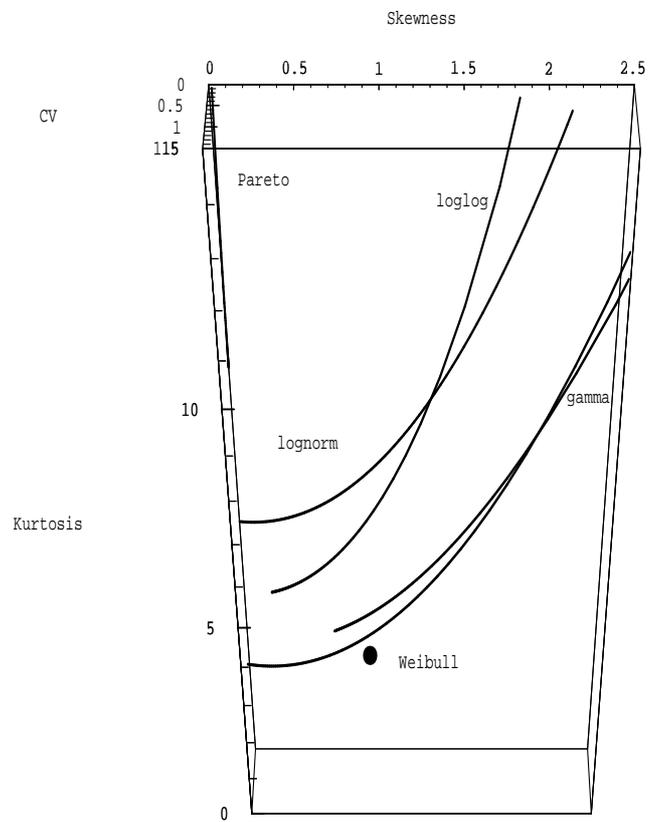
Figure 9: Kurtosis vs. Skewness vs. Coefficient of Variation [Ball Bearings at (0.52, 0.88, 3.19)]
