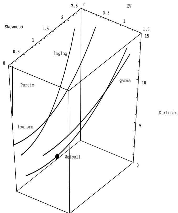
Figure 10: Kurtosis vs. Skewness vs. Coefficient of Variation, Rotated [Ball Bearings at (0.52, 0.88, 3.19)]
