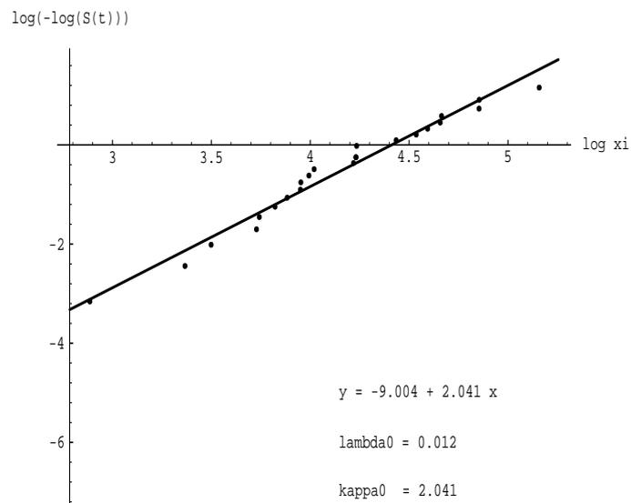
Figure 3: Weibull Plot (Ball Bearings, Weibull Fit)
