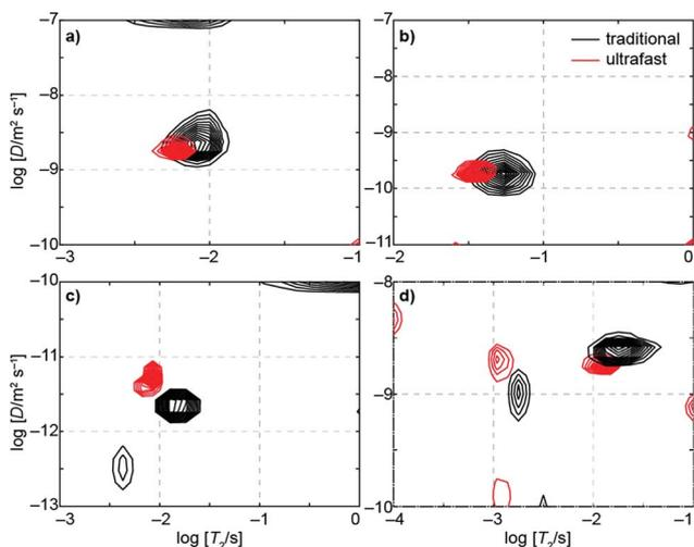
Fig. 3 Traditional (black) and ultrafast (red)  $D$ - $T_2$  correlation maps of (a) water doped with copper(II) sulfate, (b) ethylene glycol, (c) glycerol, and (d) water in 4 Å molecular sieves. Values for  $D$  and  $T_2$  for these samples are given in Table S3.†
