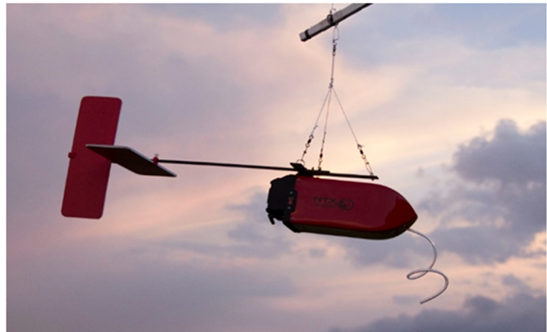
Fig. 5. (top) Schematic and (bottom) picture of the miniGAS PRO, a 1.5-kg miniature multiple-gas payload that incorporates waterproof case; GPS; and \text{SO}_2 and \text{CO}_2 , temperature, and relative humidity sensors with onboard datalogger and telemetry, designed for UAV/drone or tethered-balloon/blimp measurements.
